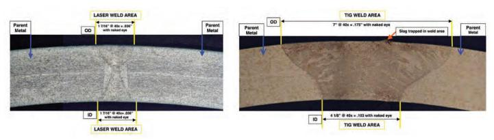
At a magnification of 40 times the actual size, the laser welded tube exhibits a narrow deeply penetrated weld compared to the wide shallow weld typical of a TIG welded stainless steel tube.
